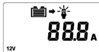
When the charging current or load current is less than 0.5Amp, the LCD will always show Min A.
