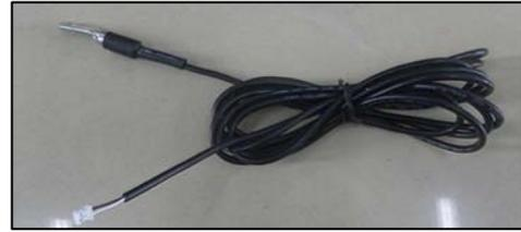
MP-3735 has both internal and external temperature sensor to detect the ambient temperature. The controller defaults to use internal temperature sensor if external temperature sensor cable is not connected. Once the external temperature sensor cable is connected, the controller will automatically switch to the external temperature sensor.
