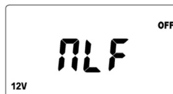
Press “menu” button once from NLF window, Window will switch to Timer1 setup interface. Press “enter” button once, you can adjust ‘Hour’ via ‘Pageup/Pagedown’ button. After ‘Hour’ setup press ‘enter’ button for confirmation and switch to ‘Minute’ adjustment. You can use ‘Pageup/Pagedown’ button to adjust it. This can be confirmed by pressing ‘enter’ button. Through ‘Pageup/Pagedown’ button, choose ‘ON’ or ‘OFF’ or ‘ON/OFF’ and then confirm by ‘enter’ button.
