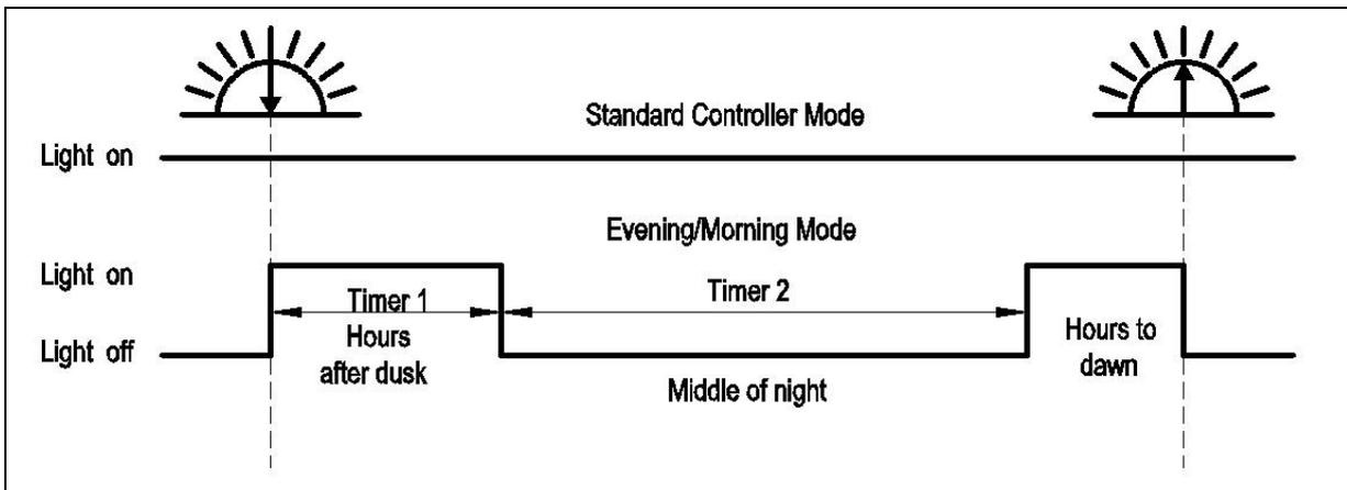
The MP-3735 recognizes days and night based on the solar array voltage. NLF will start when the PV(Voltage) < 10V for a period of time.
