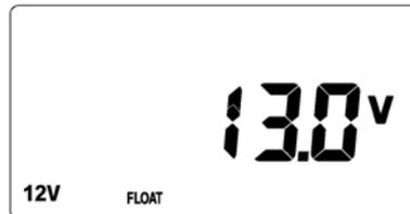
NOTE: When programming the FLOAT voltage, if you press the Pagedown button to go below 13.0V, the LCD will display OFF; meaning that the float voltage is set to ambient temperature control.
