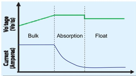
**Bulk:** This is the first stage where the battery is in a low charge state, where it receives the majority of its charge. During this stage the battery brought to about 85-95% capacity getting 100% of the available solar power.
